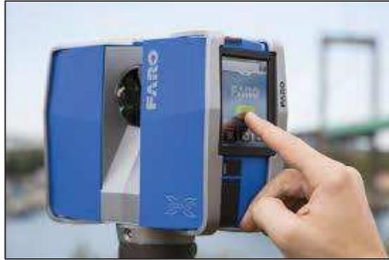
Equipement scanner Laser portable (230 x 183 x 103mm)
