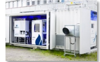
PtL-Plant with Direct Air Capture (Kopernikus Project)
